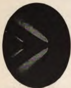
FIG. 152.—Showing the compressions and rarefactions which accompany a rifle ball in its flight.
